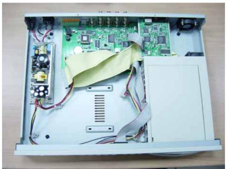
4. Please refer to the instruction from hard drive manufactory for correct jumper setting on (master /slave) mode of the hard drive, mounting the hard drive over DVR base by facing IDE interface to DVR main board. Match screw holes from bottom to bottom of hard drive and the DVR. Turn over the DVR from top to bottom side and then mounting up the hard drive by using screws from attached accessory pack as picture below:
